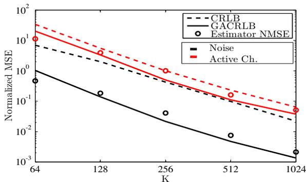
Fig. 3. NMSE for varying compression ratios.  $N = 1024$ , SNR =  $-10$  dB.
