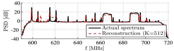
Fig. 4. Example of reconstruction of a mixed analog/digital broadcasting television band.
